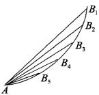
The chords  $AB_1$ ,  $AB_2$ ,  $AB_3$ ,  $AB_4$ ,  $AB_5$ , may be regarded as approximations to the tangent to the curve at A,  $AB_5$  being the most accurate approximation. The slopes of chords  $AB_1$ ,  $AB_2$ , . . .  $AB_5$  are successive approximations of increasing accuracy to the slope of the tangent at A, and therefore by definition, to the slope of the curve at A.
