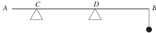
The mass of the rod is 4.4 kg,  $AC = 0.4$  m and  $AD = 2.6$  m. Calculate the magnitudes of the reactions at  $C$  and  $D$ . [7]
