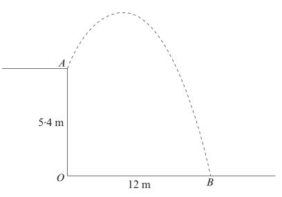
The initial velocity of the pebble is  $V \text{ms}^{-1}$  at an angle  $\alpha$  above the horizontal, where  $\tan \alpha = \frac{3}{4}$ . The pebble hits the ground at the point *B* which is at a distance of 12 m from *O*.
