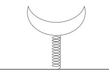
The seat is modelled as a particle P and the spring is modelled as a light spring of natural length 0.75 m and modulus of elasticity  $\lambda$ .
